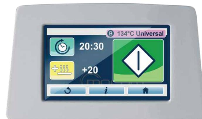
Designed to optimise the workflow, the B Futura steriliser lets users programme sterilisation and test cycle start times to take advantage of lower electricity costs at certain times of the day. This feature can also be used to prevent any overloading of electrical systems caused by simultaneous use of several devices, or simply to have the steriliser ready at the start of the next working day.
