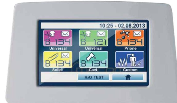
Sterilisation cycles can be selected quickly and directly via the programme-associated icons on the **touch-screen**. The display also allows the user to select the language, manage users and personalise the steriliser exactly as desired.
