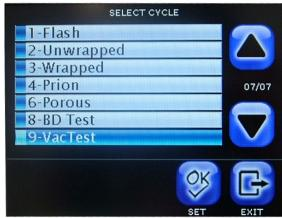
**Operation** – Operating is simple: close the door, select the cycle on the Touch-Screen Panel, and press the Start Key. The cycle will run automatically. At the end of the cycle, by pressing the 'Open Door' button on the Touch-Screen Panel, the door will automatically open.
