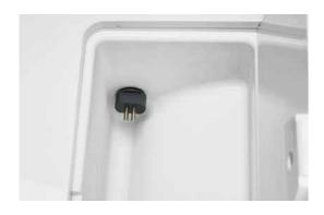
The quality of the distilled water being used is guaranteed by the conductivity sensor incorporated in the tank and an efficient warning message/alarm system. If the water is of unsuitable quality, the steriliser notifies the user with appropriate messages and prevents use of the steriliser to avoid risk of damage.
