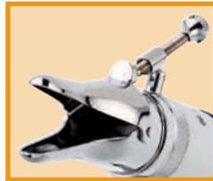
Adjustment to the desired expansion is infinitely variable by means of the knurled thumb screw.
