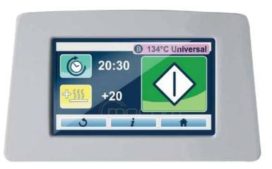
Designed to optimise the workflow, the B Futura steriliser lets users programme sterilisation and test cycle start times to take advantage of lower electricity costs at certain times of the day. This feature can also be used to prevent any overloading of electrical systems caused by simultaneous use of several devices, or simply to have the steriliser ready at the start of the next working day.
